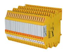
DEHNconnect DCO SD2 is an efficient surge protective device for protecting e.g. automation systems. With a width of only 6 mm, two cores are efficiently protected against surges. A HF version of the surge protective device, which is ideally suited for high transmission rates, is now available.
