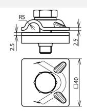
Multipurpose connecting clamp with spring washer for universal use as cross, T and parallel clamp; two-piece design. Tested for lightning current carrying capability up to 200 kA (10/350 µs).
